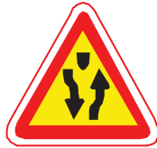
Divided Road Begins. Posted before the beginning of a divided roadway. Vehicles are to remain right of the road divide.
