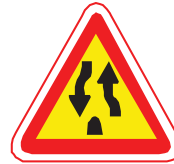
Divided Road Ends. Posted at the end of a divided roadway. Oncoming traffic ahead.
