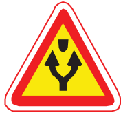
May Travel Either Lane. Posted before an obstacle in the road. Vehicles proceed either side of the obstacle.
