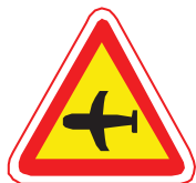
Low-flying Aircraft. Posted near areas where aircraft fly at low altitudes (for example, airports).
